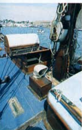
Left: Nausikaa's liferaft stowage dominates the yacht's foredeck, and holds an Avon Redstart and the air bottles to inflate it. The deck prism lights the heads. The pitch pine deck is covered with Trakmark.
